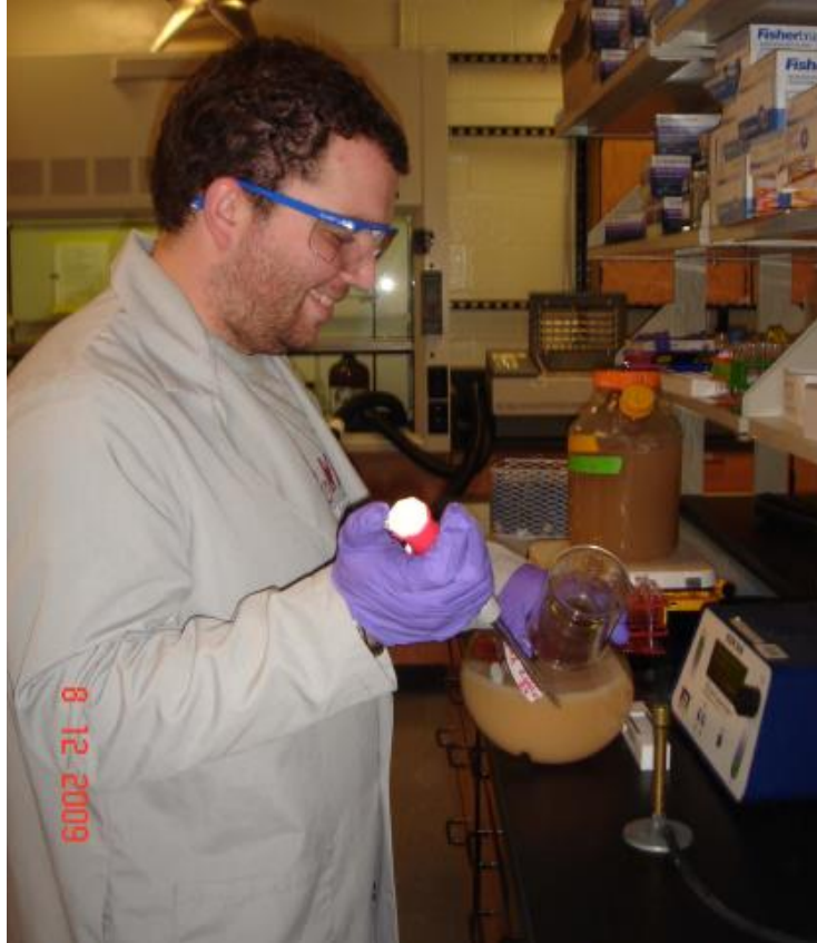
Figure 4.10 Transferring oil-rich media to Teflon™ cuvette for electroporation experiment
