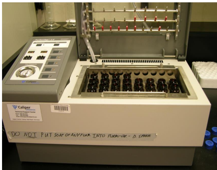
Figure 4.15 TurboVap loaded with amber vials to evaporate chloroform
