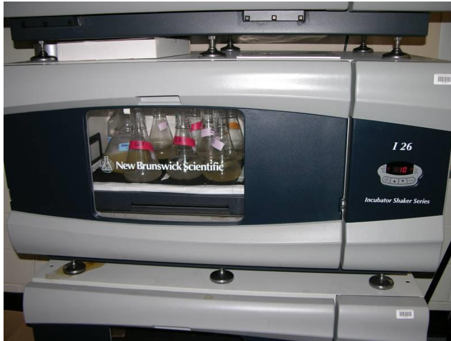
Figure 4.6 Inoculated bottles in constant motion incubator
