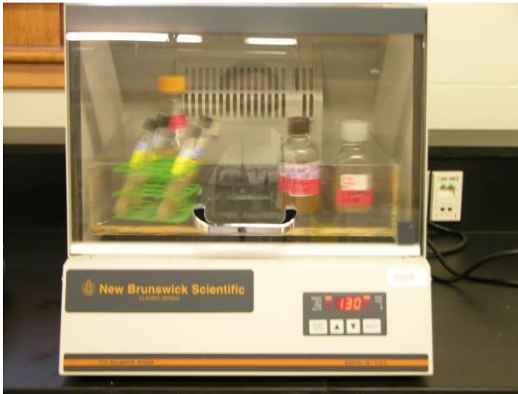
Figure 4.3 Agar and growth media in a New Brunswick Scientific constant motion incubator
